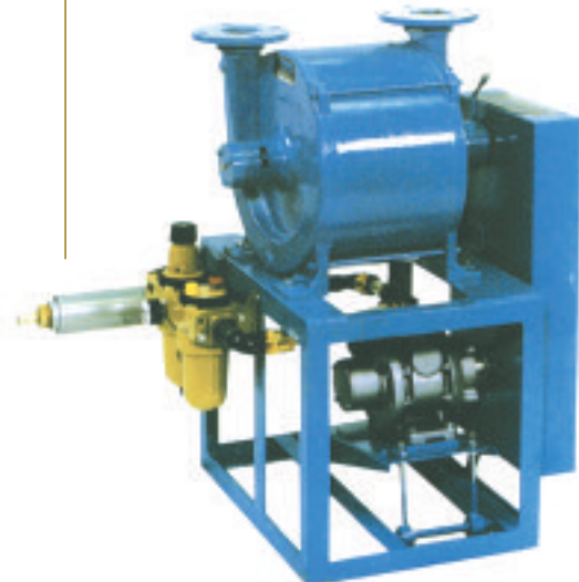
6X5 Turbo Blower driven by an air powered motor.
